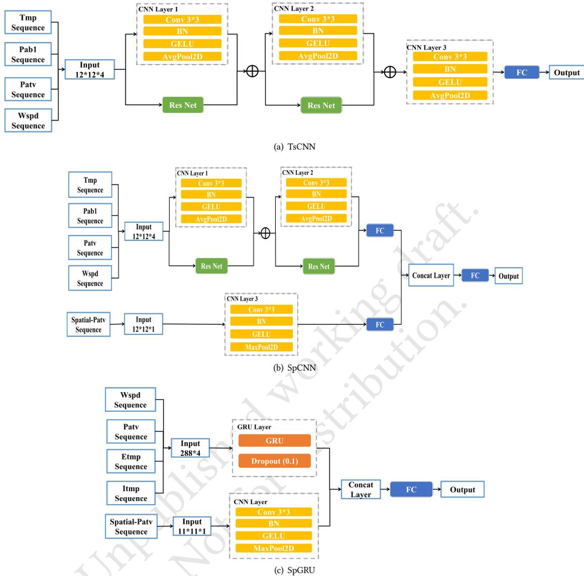
Figure 2: Deep learning models in proposed framework. (a) CNN model with multichannel time series (TsCNN). (b) CNN model with spatial-temporal information (SpCNN). (c) GRU model with spatial-temporal information (SpGRU).
