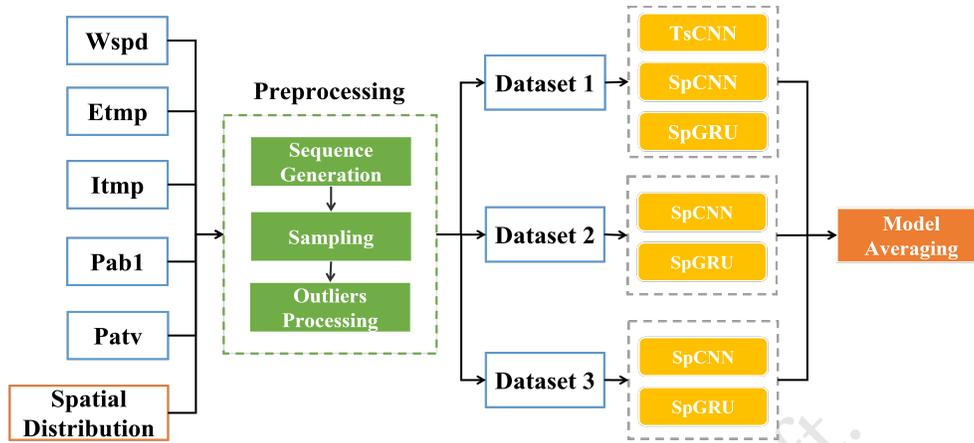
Figure 1: Our proposed framework for the spatial dynamic wind power forecasting
